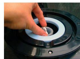
Remove the cotton located in the polypropylene receptacle.
