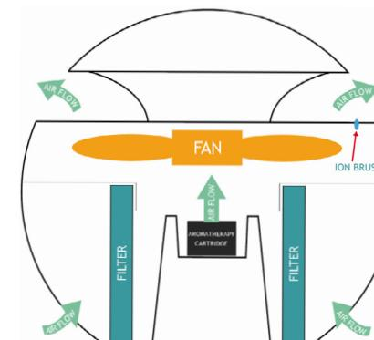
The fan draws air through the openings in the unit. The air is purified through a E11 type particle filter which retains the pollen, bacteria and small particles.
