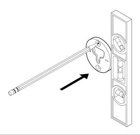
Pre-drill pilot holes into a stud using a 9/64" drill bit. Place the bracket against the wall with the small arrows pointing up, and secure it to the wall with 2 long wall bracket screws (included) and a power drill or Phillips-head screwdriver.
