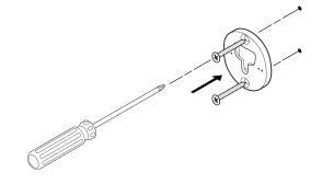
Remove the screw from the mount assembly. Rotate the mount 180 degrees so the screw holes are facing up, then reattach the screw to the mount assembly.
