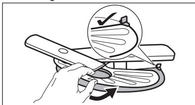
7. Reassemble the filters (B) and (C).
