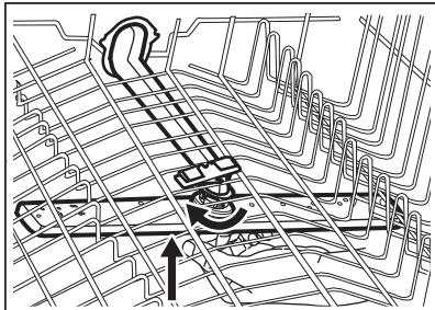
3. Wash the spray arm under running water. Use a thin pointed tool, e.g. a toothpick, to remove particles of soil from the holes. Run water through the holes to wash soil particles away from the inside.
